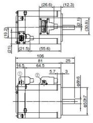
① Encoder connector 2 Motor/Brake connector
